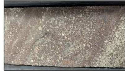
Figure 2 (b). Massive sphalerite and pyrite from 230 m downhole.
