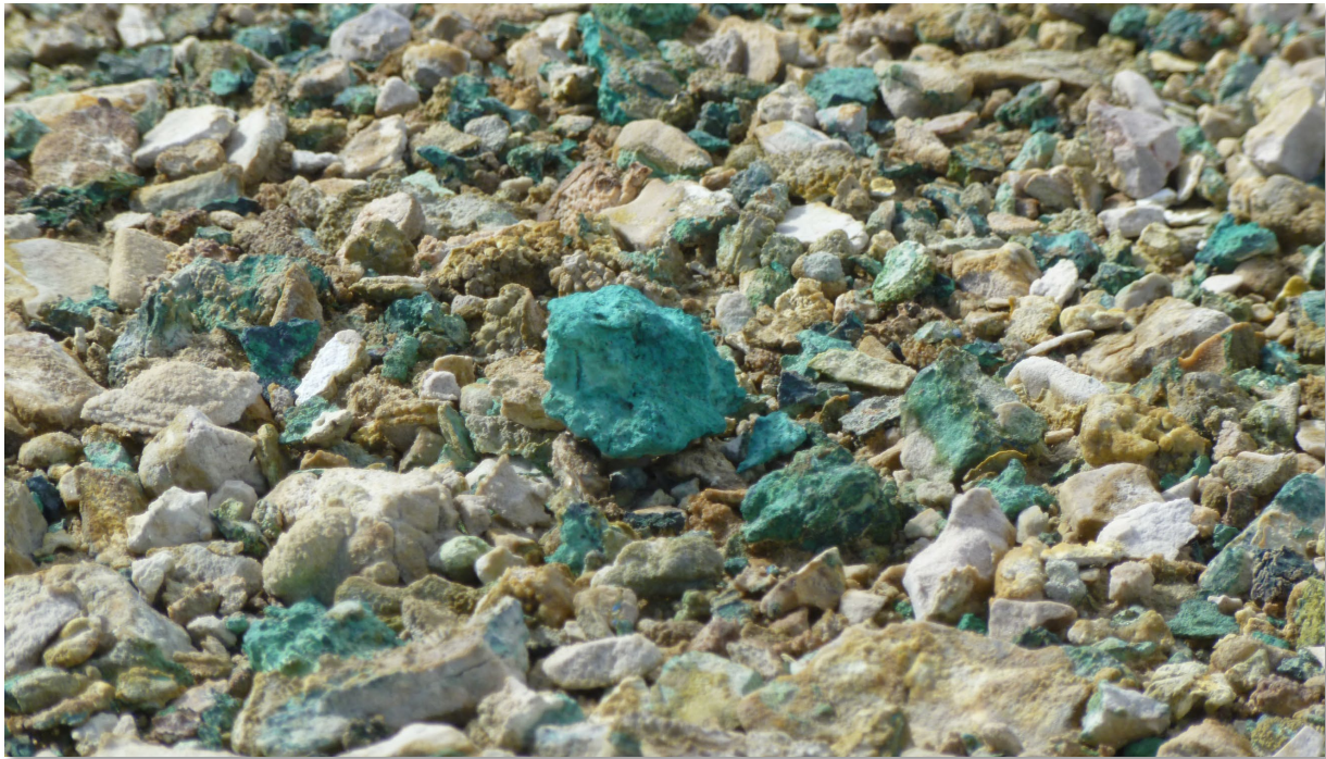
Figure 2: Chalcocite (with some malachite alteration in this photo) is extensively exposed at surface at Storm and suggests potential ‘leakage’ sourced from a large sediment-hosted copper system below.
