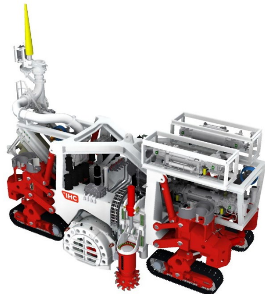
Arctic Canadian and IHC Mining’s Underwater Mining Crawler for the Underwater Remote Mining System. The crawler will help recover diamond-bearing kimberlite ore from deep open pits at the Ekati Diamond Mine, in the Northwest Territories of Canada.
