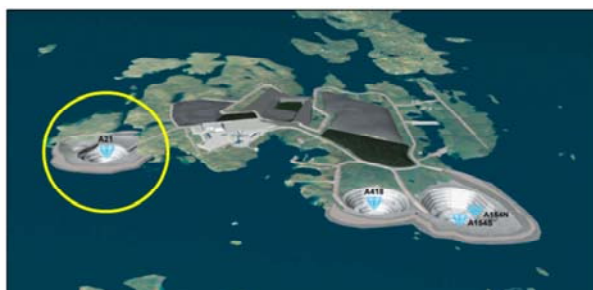
A21 is under the lake, and will be developed with similar dike technology as shown around the A418 and A154 deposits. Courtesy: Diavik Diamond Mines Inc.
