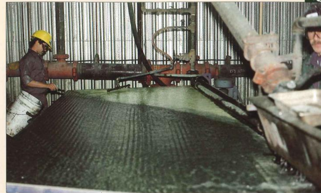
▲ A Shaking Table Uses Gravity to Separate the Gold. The Operator is collecting the gold grains at the end of the Table.
