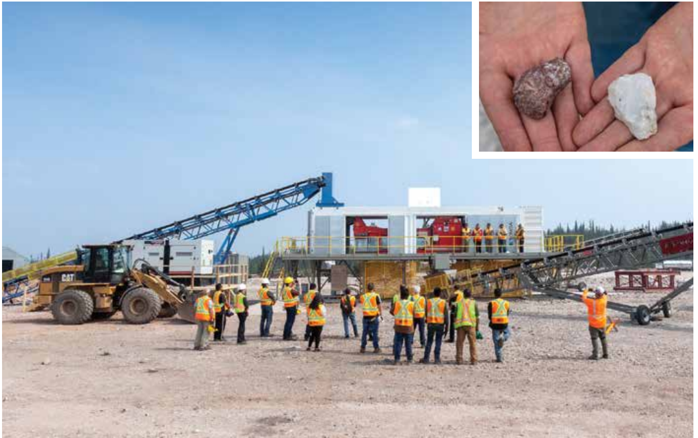
Above: The TOMRA ore sorter at Nechalacho, which uses X-rays and puffs of air to separate the ore from the quartz.
