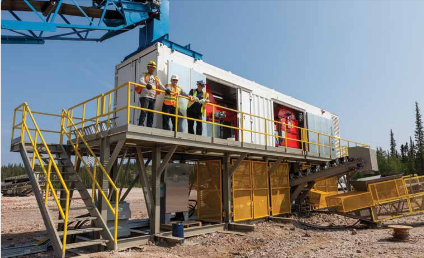
The TOMRA computerized ore sorter at Nechalacho uses X-ray and air jet technology to separate the bastnaesite ore from the host quartz rock.
