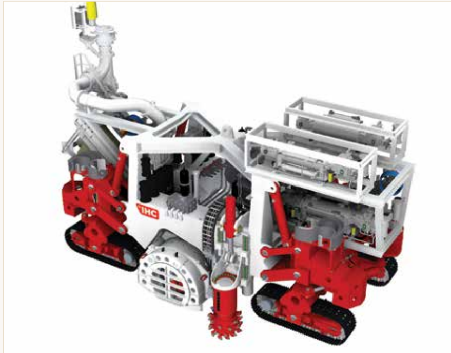
The URM – Underwater Remote Mining – a remote-operated “bottom crawler” deployed from a floating platform on the lake surface, proposed for use at Ekati.
