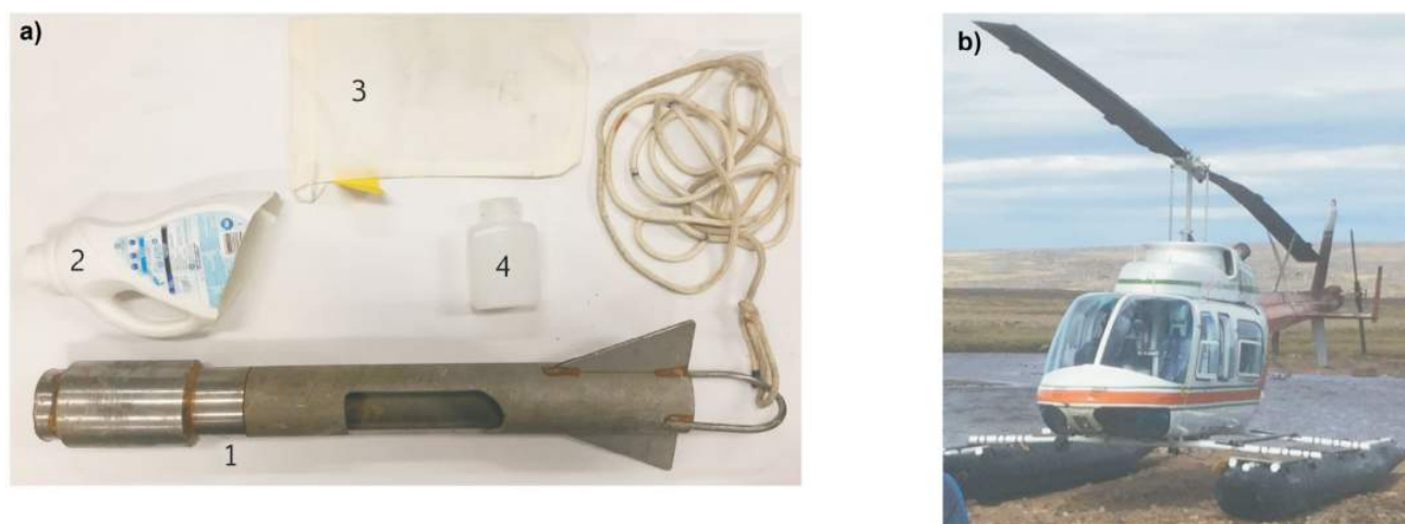
Figure 6: a) Field gear used for lake sediment and water sampling: 1) torpedo-like lake sediment sampler, with 30 m rope; 2) plastic cup for extracting the lake sediment core from the sampler; 3) cloth bag for sample; 4) 250 ml sampling bottle—sample is split into two 60 ml water samples (filtered with 0.45 µm filter). Also used for lake sediment and water sampling is the YSI Inc. Professional Plus multiparameter water meter (Figure 5a-2) and the iPad for navigation and recording site-specific field observations (Figure 5a-9). b) Helicopter on fixed floats used for lake sediment and water sampling survey.
