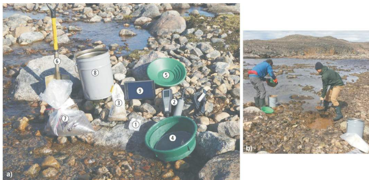
Figure 5: a) Field gear used and samples collected at a typical bulk stream sediment and water site: 1 ) two 60 ml water samples (filtered with 0.45 µm filter); 2 ) YSI Inc. Professional Plus multiparameter water meter; 3 ) silt-sized stream sediment sample (~2 kg wet); 4 ) #10 mesh (2 mm) sieve; 5 ) pan; 6 ) steel shovel; 7 ) bulk stream sediment sample (>12 kg of ≤2 mm sediment); 8 ) bucket lined with prelabelled sample bag (not yet stretched tightly about the bucket opening); and 9 ) iPad used for navigation and recording site-specific field observations. b) Typical bulk stream sediment and water sampling site.
