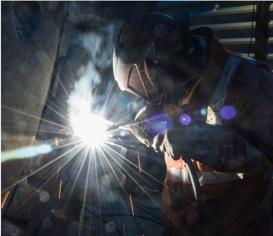
Left: Rylan Stauder, a Paul Bros Nextreme employee from Yellowknife, welds a piece of track for one of the massive mining shovels at Gahcho Kué Mine.
