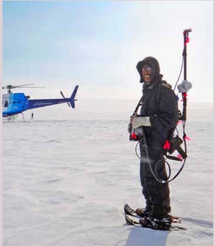
Robert Joamie conducting ground magnetics, Chidliak project Courtesy of Peregrine Diamonds
