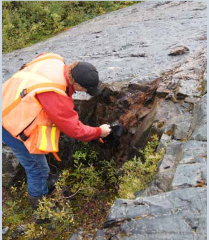
Geologist examining uraniumiferous veins with a scintillometer, Angilak Courtesy of AANDC
