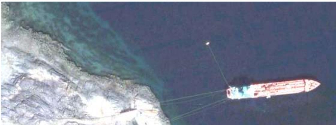
**Google Earth Image of Sealift Tanker Discharge at Iqaluit Inuit Head Pipeline Header.**
