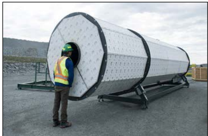
The composter vessel at the Ekati mine
