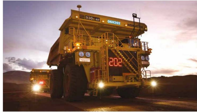
Autonomous Haulage System in operation in the Pilbara, Western Australia
