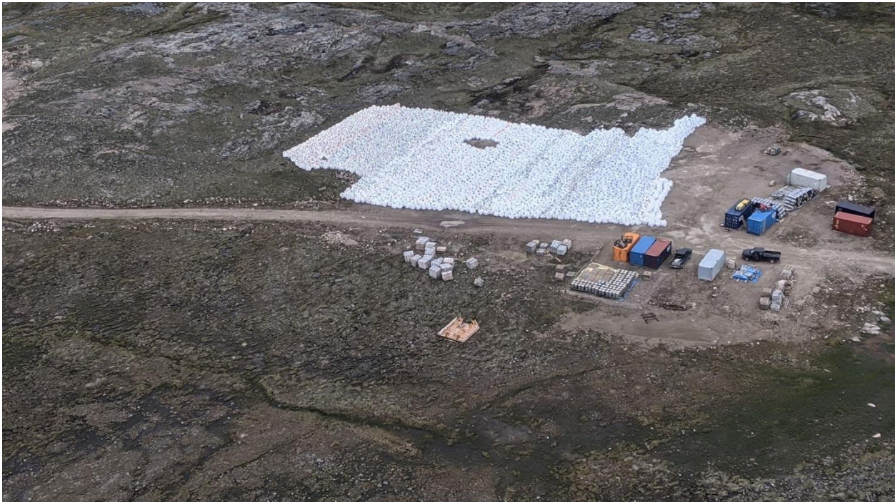
2500 mega-bags of the Q1-4 kimberlite at the NAR Laydown Area near the Naujaat town quarry. The bags will be loaded on to the September sea lift for ocean transport to Montreal and then on to Saskatoon by truck for processing at the SRC.
