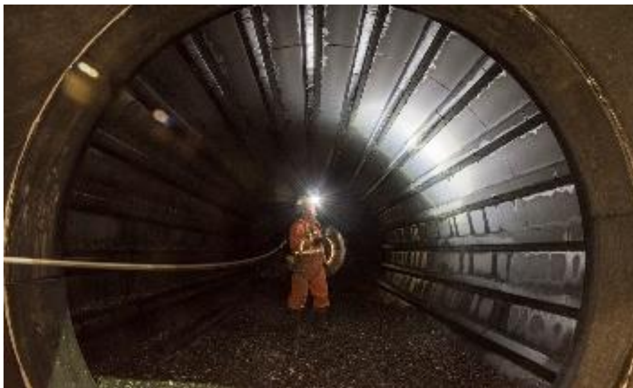
A Gahcho Kué mine worker inspects a scrubber, a rotating drum used to help break down ore. De Beers photo
