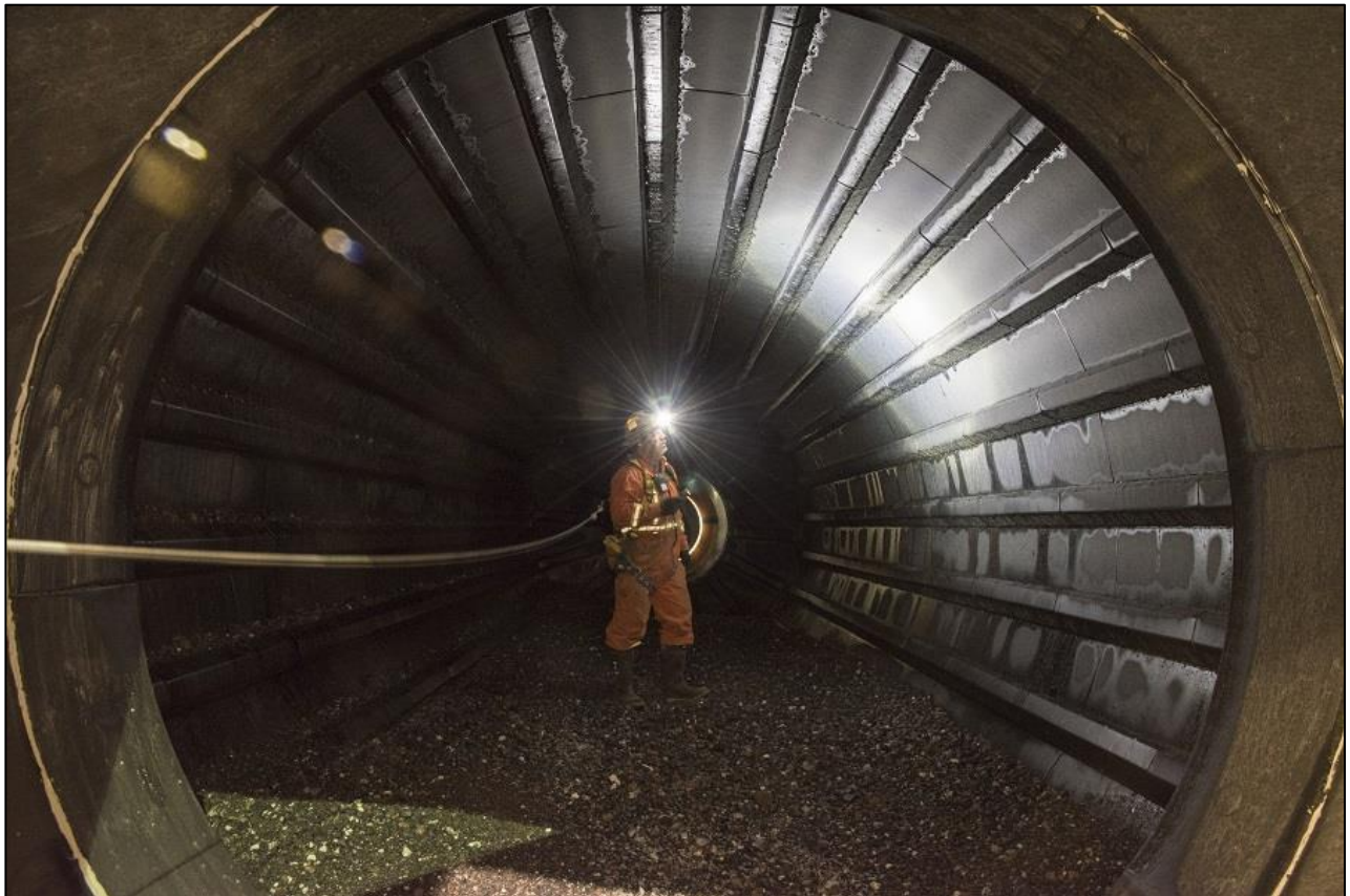
A worker inspects a scrubber in the Gahcho Kué mine process plant. De Beers/Mountain Province photo
