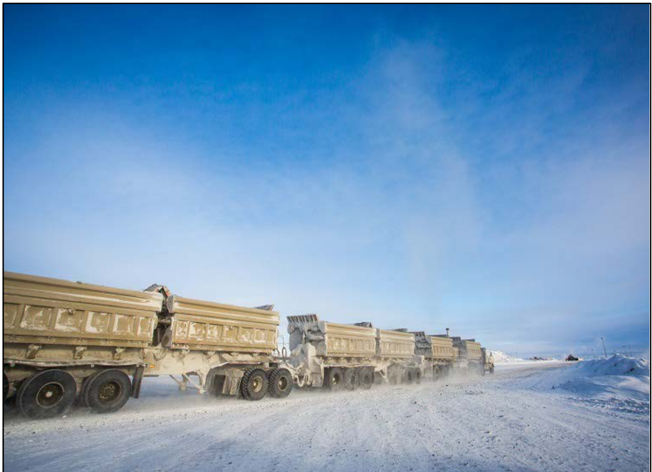
At Ekati, to improve fuel efficiency and reduce emissions, Dominion uses road trains for ore haulage.
