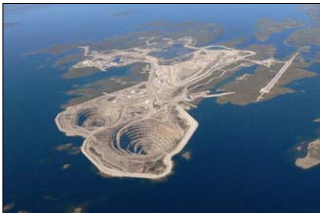
New dike technology allows Diavik to mine diamonds from the lake bottom, and will let them return it as fish habitat later.
