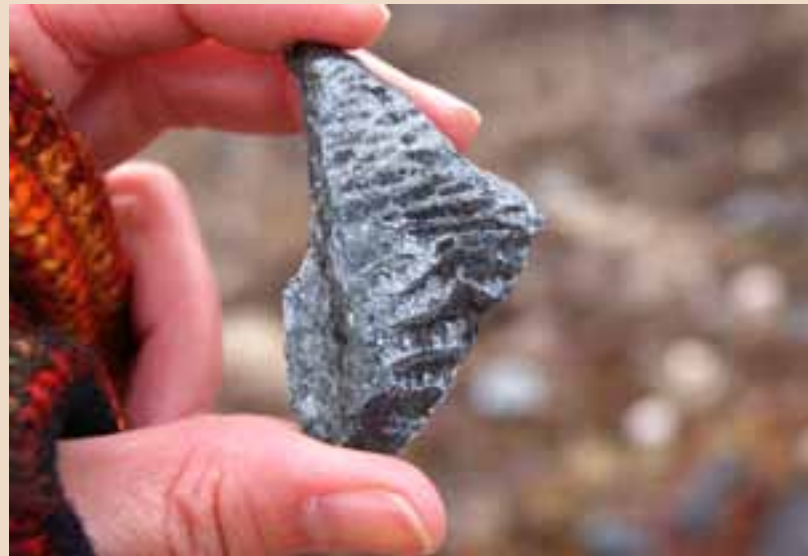
Crenulation cleavage in specular hematite, Deposit No. 4, Mary River Courtesy of AANDC
