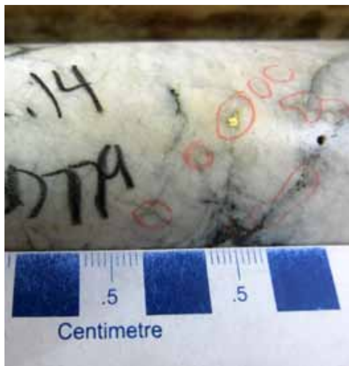
Drill core with visible gold from Hope Bay Courtesy of Hope Bay Mining
