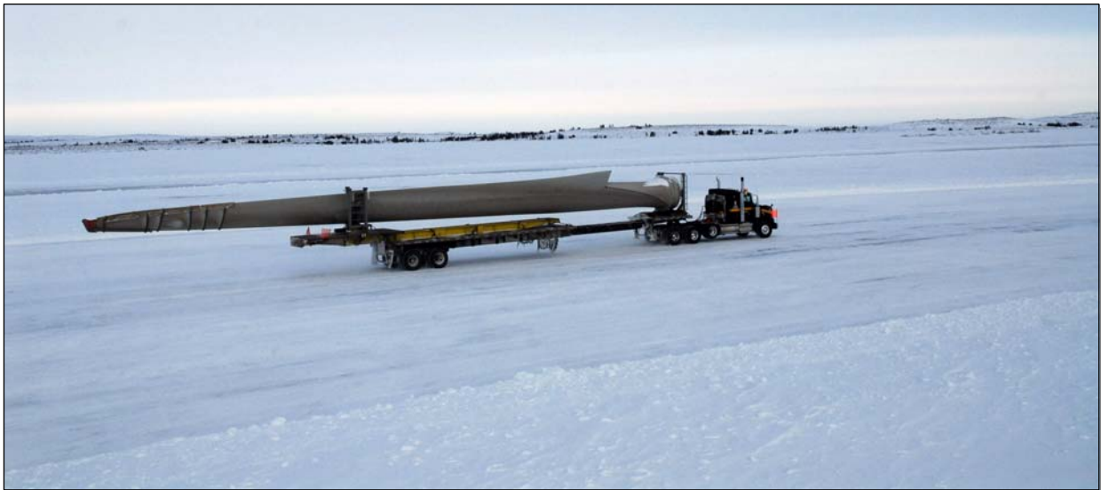
Custom-designed trailers were required to truck Diavik's 33-metre long epoxy-resin wind turbine blades, the longest loads ever shipped over the ice road.
