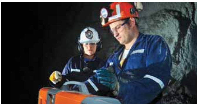
Sirovision is a geology / geotechnical mapping and analysis system that generates accurate, scaled 3D images of rock faces from stereo photographs taken in open-pit and underground environments. Photo courtesy of CAE Mining.
